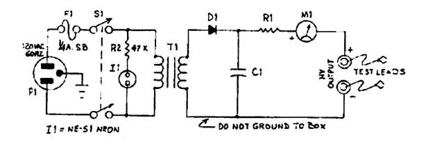
THE CIRCUIT: The figure shows all there is to this nifty addition to your workbench. In my unit, transformer T1 is a small H.V. transformer out of an old oscilloscope. It furnishes about 1.600 vac. at 2 or 3 milliamps. Other transformers can be used for T1 so long as they provide somewhere between 1.000 and about 3.000 vac. Current demand is very low in this application. So for conservation and safety reasons,
